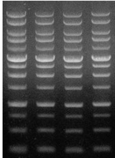
**Figure 2.** PCR product DNA fragments ranging from 250 bp-10 kb were extracted using the GenepHlow™ PCR Cleanup Kit (lane 1, 2, 3). The purified DNA concentration from a 50 µl eluate was confirmed by spectrophotometer and analyzed by electrophoresis on a 1% agarose gel.
